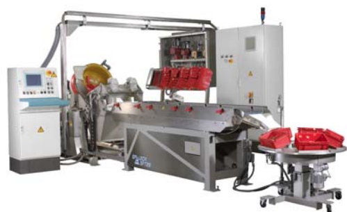
Picture 5: Fully automated Spaleck Finish gold and silver coin blank installation Z33-SFT
